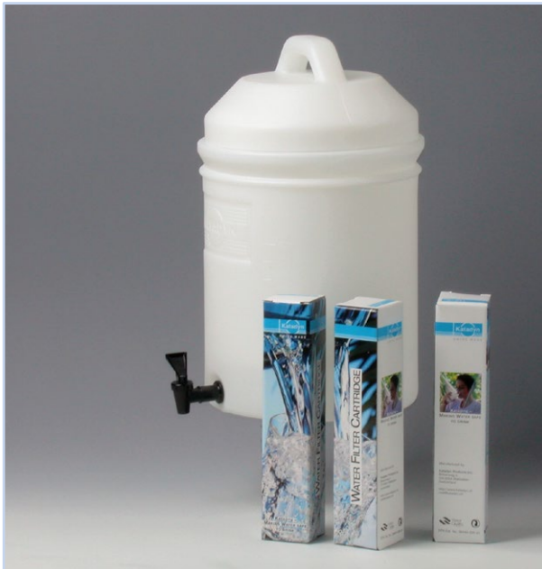
Art.Nr.: 62070 Water filter, KATADYN including 3 filter candles, approx 4.5 litres/h. The drop filter consists of two tanks. Fill the water into the top tank. It then drops slowly through the three ceramic cartridges into the lower tank. A run-off tap is mounted in the floor of the lower tank (max. 10 litres).
