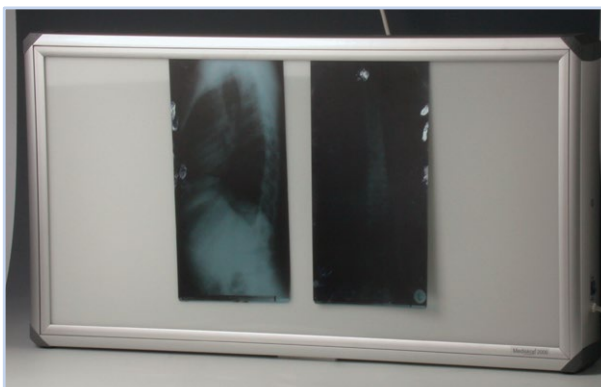
Art.Nr.: 40170 X-ray viewer screen approx. 80 x 43 cm, wall mounted without blinds, external housing approx. 106 x 11 x 60 cm (W x D x H), 120 W, approx. 10,300 Lux, approx. 6500 Kelvin, Mains supply 220 V, Weight approx. 22 kgs
